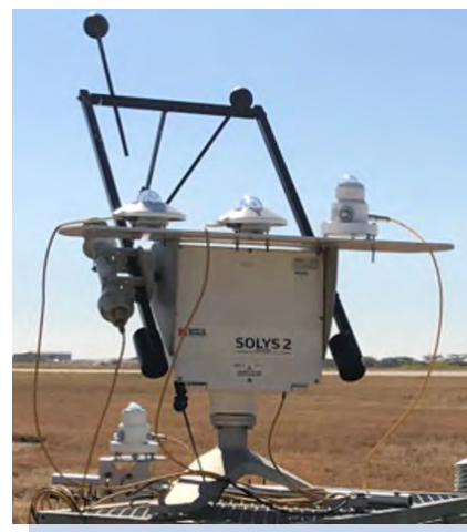
Figure 1: Configuration of a radiometric station with an unshaded pyranometer at the centre
